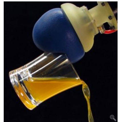
Researchers at the University of Chicago, Cornell University and iRobot developed the Universal Robotic Gripper based on the jamming of granular material. The gripper will among the topics discussed at a workshop on “Frontiers in Pure and Applied Jamming,” which will meet Oct. 26 to 28 at UChicago and the Illinois Institute of Technology.
